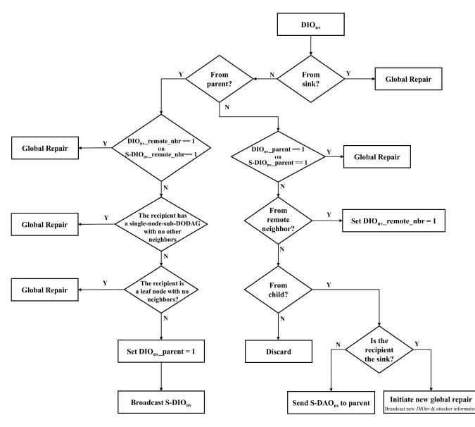
FIGURE 2. An overview of the DIOnv processing procedure.
