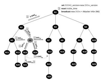
**FIGURE 6.** Example of a simple VN attack scenario with a single attacker (N6).
