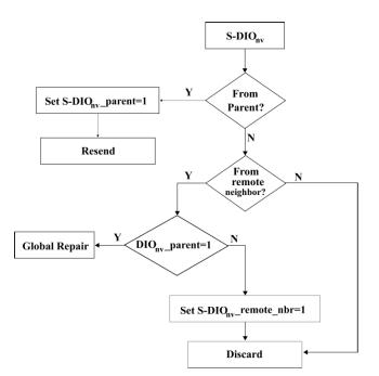
FIGURE 3. An overview of the S-DIO<sub>nv</sub> processing procedure.
