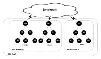
**FIGURE 1.** An example of an RPL network of two RPL instances with varying DODAGs.
