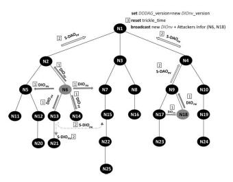
FIGURE 7. Example of a composite VN attack scenario with two attackers (N6 and N18).
